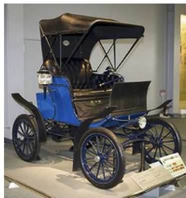
The Baker electric car could travel up to 80 kilometres on a single charge.
