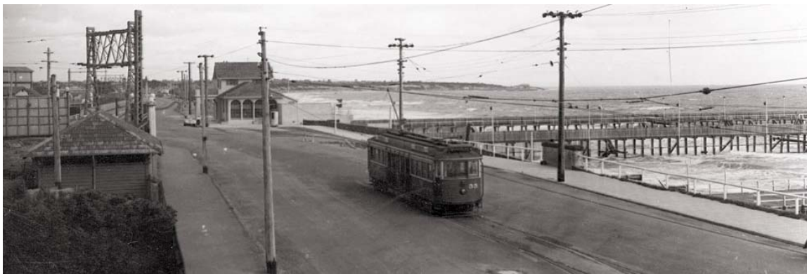
"Tram 33 is seen at the Brighton Beach terminus of the 5' 3" gauge VR ELECTRIC Street Railway that ran from St Kilda station and was opened in 1906. On Jan. 1 1957 the line was cut back to Middle Brighton crossover. The last section of this street railway, Middle Brighton to Elwood depot, closed June 1957. The brick parapet seen to the right of the tram locates the end of a short tunnel section of rail line that ran from Brighton Beach 'luggage room' (goods shed) along the pier seen on the right. Photo circa 1930's" Ref: Ref: Mark Bau's VR Website www.victorianrailways.net/index.html
